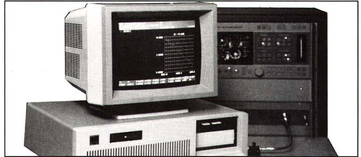
IBM AT compatible software permits calibration of test fixtures for real-time de-embedding.
