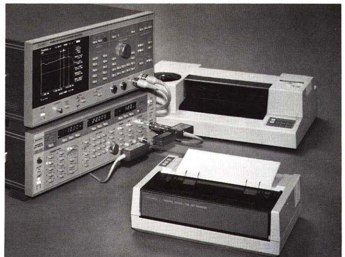
Hard copies of all displayed test data and parameters can be made on a dot-matrix printer or GPIB plotter while measurements proceed.
